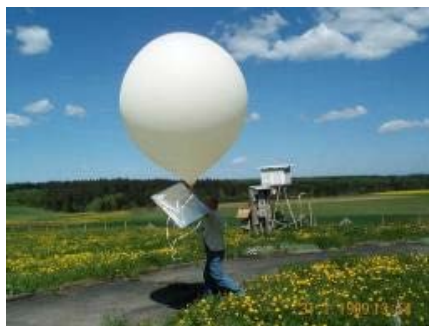
Balon meteorologic cu reflector
